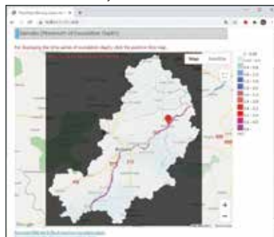
Maximum flood inundation depth map of the 2018 flood event in the Bamako area of the Niger basin simulated by the national WEB-RRRI model.
